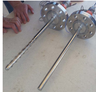
Figure 2 - Thermowells used to 'sample' from the centerline within the 12" pipeline
